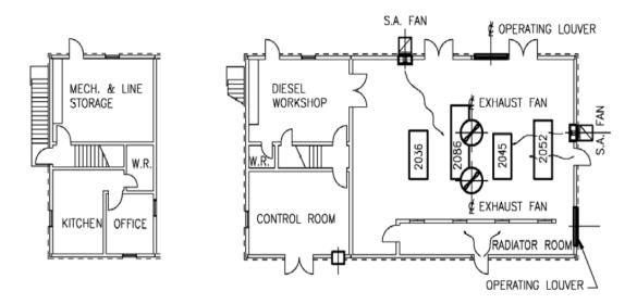
Figure 2: Cartwright Plant Ventilation Existing Arrangement
